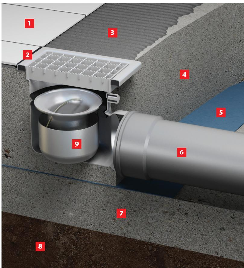
**Fixed height gully with horizontal outlet with internal FAT in ground slab with a tile floor finish connecting into stainless pipe.**
