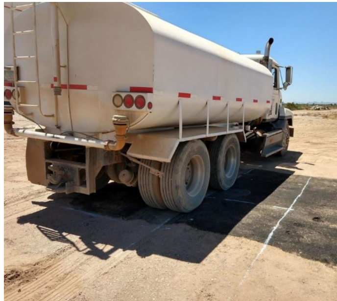
Fully loaded water truck used in full scale testing of the underground geocellular tank.
