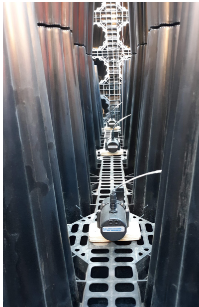
In-situ tests used wire potentiometers to measure vertical and lateral pressures.
