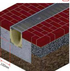
1. Grate should be 3mm below pavement surface.
