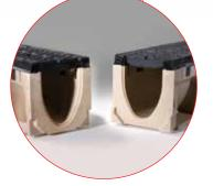
Interconnecting end profiles allow easy and effective joining of channels. SF Sealant Groove - a groove is cast into both ends of every channel. The combined groove allows for a bead of appropriate flexible sealant to be inserted at joints, if required.
