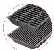
Ductile iron grates – rated up to AS 3996 load class G (approx. 30 tonne wheel load) heavy duty ductile iron Slotted or Intercept Heelsafe® Anti-Slip grates.
