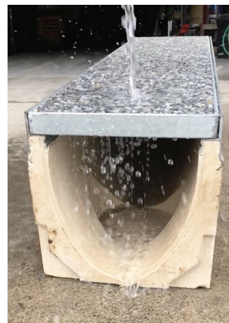
EcoPanel has been hydraulically tested
