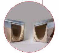
Interconnecting end profiles allow easy and effective joining of channels. SF Sealant Groove - a groove is cast into both ends of every channel. The combined groove allows for a bead of appropriate flexible sealant to be inserted at joints, if required.
