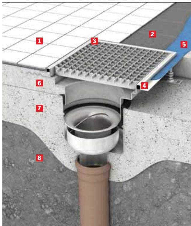
**ACO tray channel telescopic type – gully with location flange (Tiled floor)**
