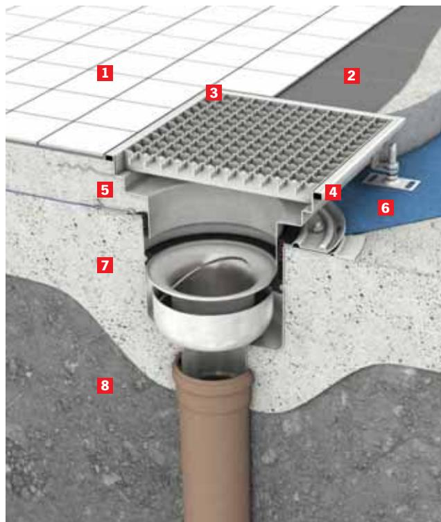
**ACO tray channel standard type – gully with location flange (Resin floor)**
