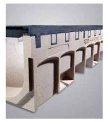
Profiled side walls provide channel body strength and anchoring to surrounding concrete. Arched side pocket profiles provide superior structural rigidity.
