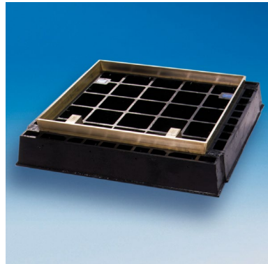
Decorative edge can be attached to the cover and frame for aesthetic areas and adds 12 or 40mm to overall height to allow for use of tiles or pavers
